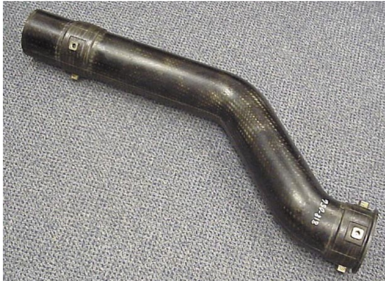
This 4-foot aircraft engine cooling duct was produced using the solvent-assisted Resin Transfer Molding process.
