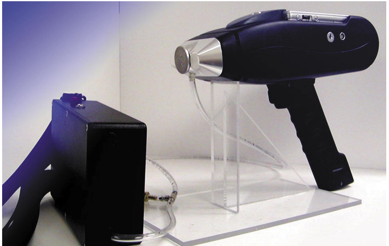
The TRACeR tags and detects unique elemental codes for material analysis and identification.
