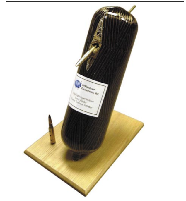
This image shows one of HyPerComp Engineering, Inc.'s test cylinders. Applications for the company's hybrid pressure vessels include fire safety and the automotive industry.
