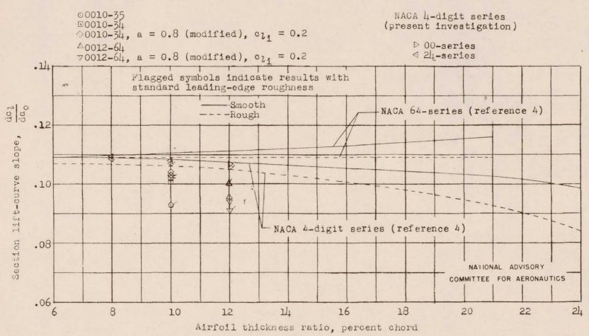
Figure 19.- Section lift-curve slopes of several modified NACA four-digit-series airfoil sections, both with and without standard roughness, as compared with those of a number of NACA 64-series and NACA four-digit-series airfoil sections. R = 6.0 x 106.
