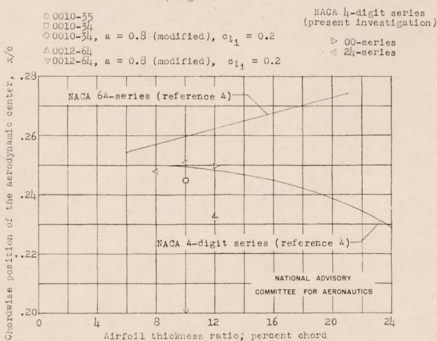
Figure 21.- Chordwise position of the aerodynamic center of several modified NACA four-digit-series airfoil sections as compared with those of a number of NACA 64-series and NACA four-digit-series airfoil sections. R = 6.0 x 106.
