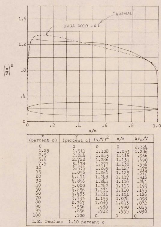
Figure 2.- NACA 0010-64 basic thickness form.
