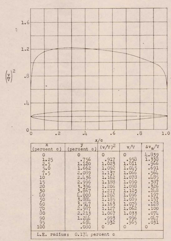
Figure 1.- NACA 0008-34 basic thickness form.
