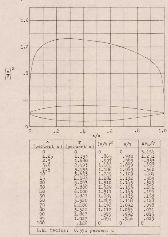
Figure 7.- NACA 0012-34 basic thickness form.
