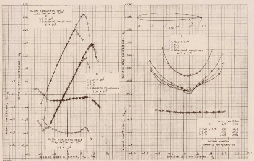
Figure 14.- Aerodynamic characteristics of the NACA 0012-64, a = 0.8 (modified), c21 = 0.2 airfoil section, 24-inch chord.
