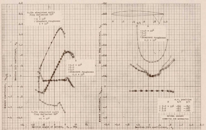
Figure 11.- Aerodynamic characteristics of the NACA 0010-34, a = 0.8 (modified), c21 = 0.2 airfoil section, 24-inch chord.
