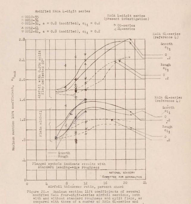
NACA four-digit-series airfoil sections.  $R = 6.0 \times 10^6$ .
