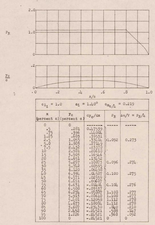
Figure 9.- Data for NACA mean line a = 0.8 (modified).
