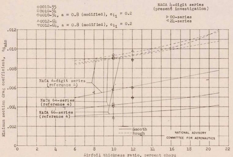
Figure 18.- Minimum section drag coefficients of several modified NACA four-digit-series airfoil sections, both with and without standard roughness, as compared with those of a number of NACA 6-series and NACA four-digit-series airfoil sections.  $R = 6.0 \times 10^6$ .
