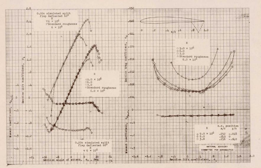
Figure 17.- Aerodynamic characteristics of the NACA 2410 airfoil section, 24-inch chord.
