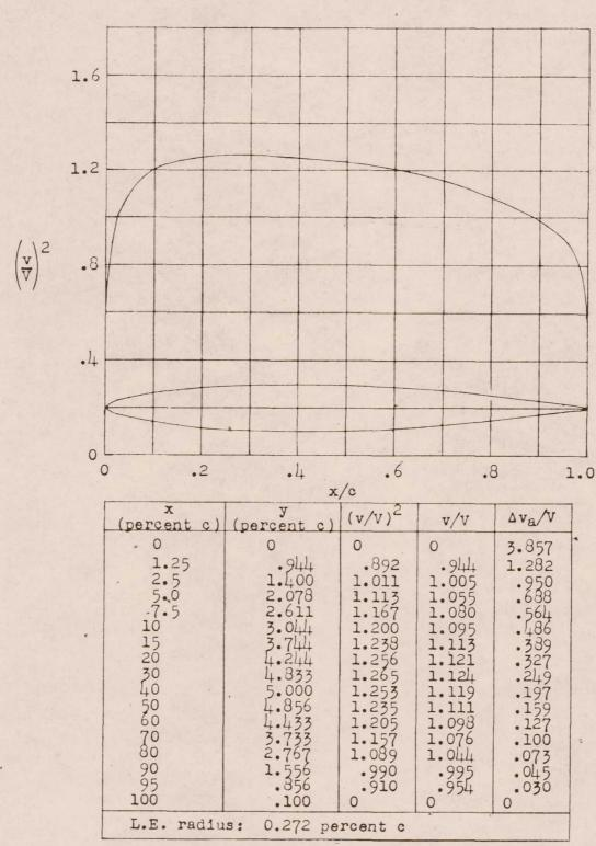
Figure 5.- NACA 0010-34 basic thickness form.
