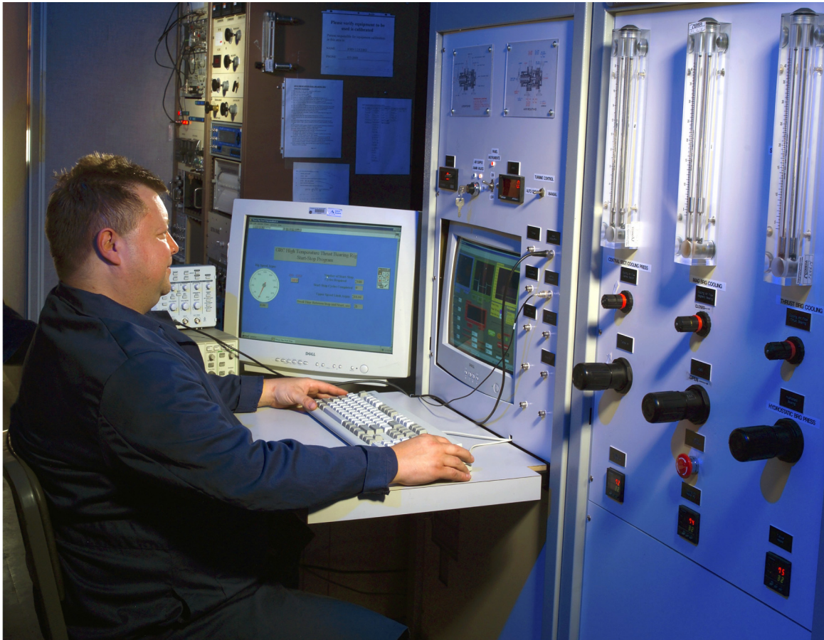
Figure 11.—Instruments and controls. A photo of the two control consoles. The left console has the computer CRT and some LED instrumentation. The right console has six air control valves and three flow meters.
