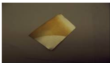
Figure 2. A section of the aluminum canister thermal shield post-flight, showing areas with and without brown discoloration.
