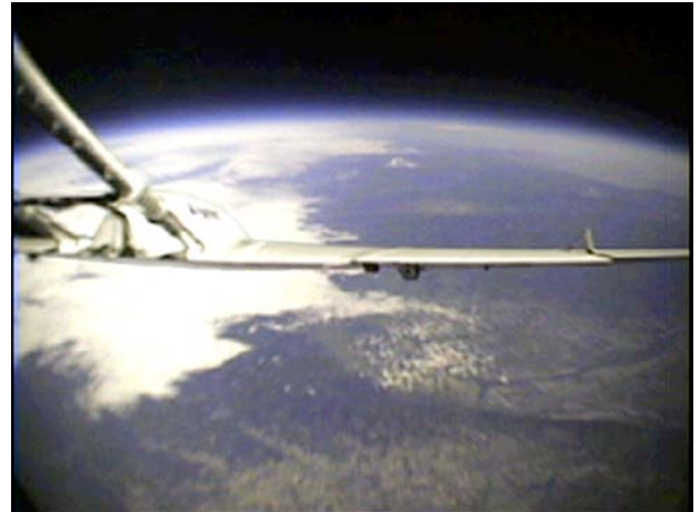
Figure 3. Video still from the successful deployment of a half-scale model of ARES at Mars-relevant atmospheric pressure above Oregon, USA (see http://marsairplane.larc.nasa.gov/multimedia.html for full sequence).
