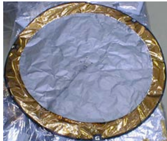
Fig. 1. 80 cm diameter of circular foil before launch.
