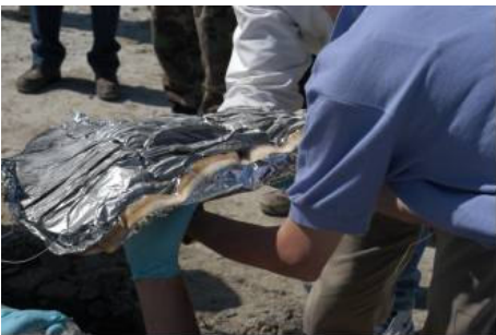
Figure 3. The molybdenum-coated foils are removed from the SRC lid in the field at UTTR.
