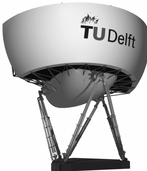
Figure 1.1. Six-Degree-of-Freedom Hexapod Motion System. Delft University, The Netherlands.
