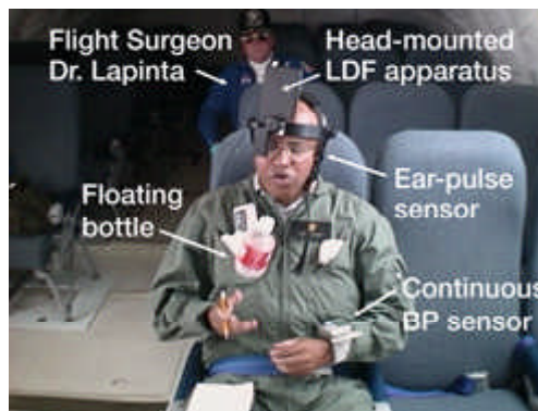
Head-mounted LDF instrument on a volunteer subject monitors ocular blood flow in 0g onboard the KC-135 aircraft.
