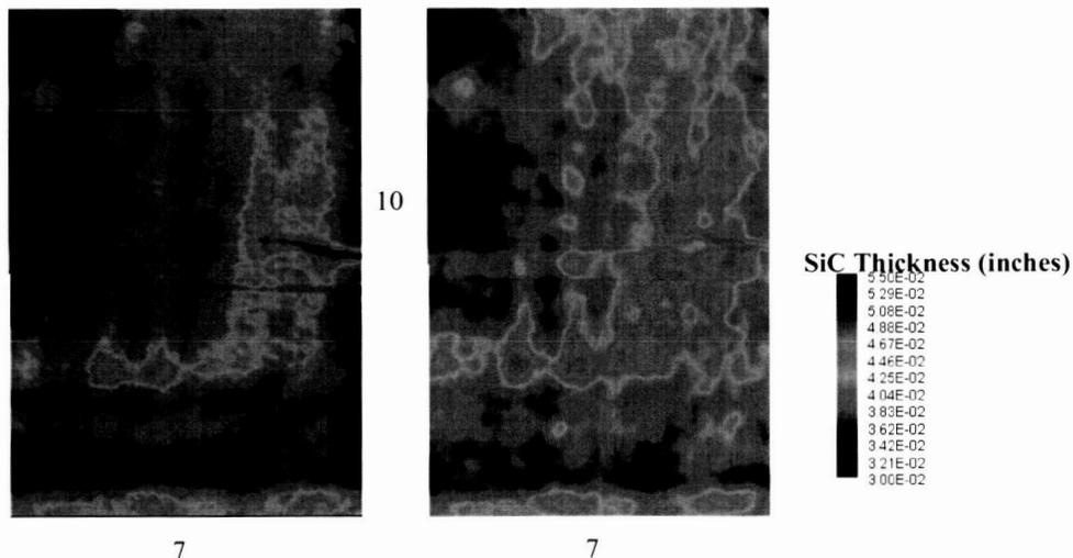
**Figure 4. Eddy Current NDE images from RCC specimens.** The left hand figure is an image from an eddy current scan of an RCC test panel showing the conductivity of the panel. The red mark on the right hand side of that panel is from a crack in the carbon-carbon. The right hand figure is an image of the eddy current probe "lift off" which corresponds to the SiC thickness.
