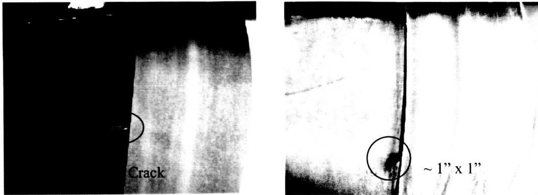
**Figure 2. Thermography images from an RCC Shuttle panel 6L.** *Figure on the left shows the thermography image of Shuttle hardware that was impacted, generating a crack visible on the surface. The right panel shows a similar thermography image after the data was post processed by PCA. This analysis shows more damage detail.*
