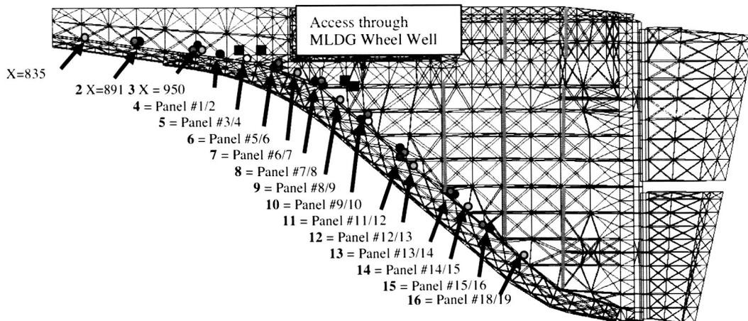
**Figure 12. Shuttle tests.** The figure shows the location of a series of sensors for a test of the sensors' response to controlled excitations.
