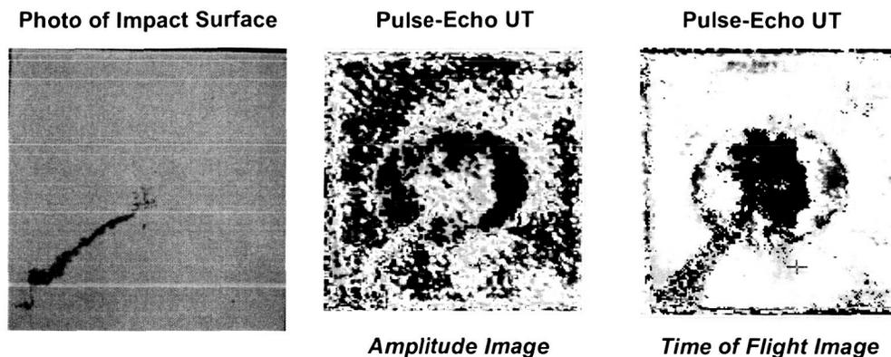
**Figure 7. Ultrasonic backscatter images of damage in RCC.** *The left hand figure is a photograph of a RCC panel with a visible crack. The middle panel is a "C-Scan" image of the amplitude of the ultrasonic signal from the interior of the panel. The right panel is a "C-Scan" image of the time of flight of the signal to the internal damage. That signal is related to the depth of damage.*
