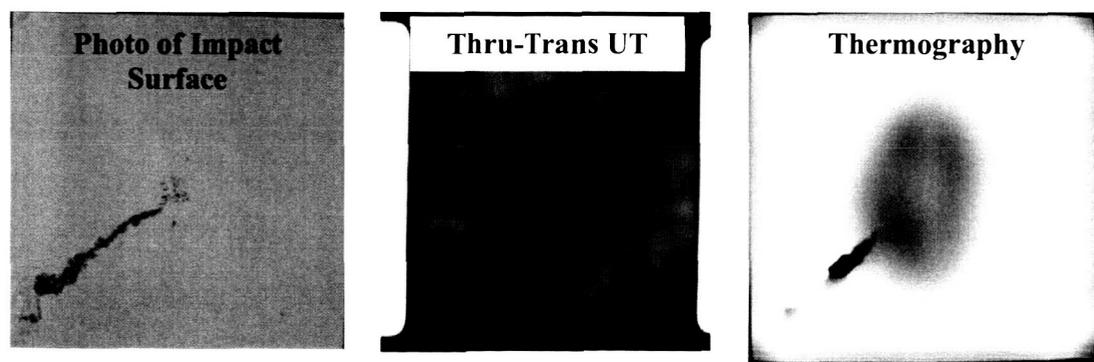
**Figure 1. NDE images from an RCC impact coupon.** *The left figure is a photograph of an impacted RCC test panel with a visible crack. The center view is a thru transmission ultrasound image. The panel to the right shows a thermography image. The ultrasonic and thermography images illustrate the hidden damage within the RCC panel.*
