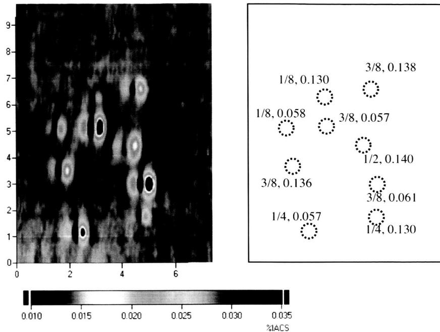
**Figure 5. Inspection results and actual flaw diameter, depth from inspection surface.** *The right hand figure is a schematic of the pattern of flat bottom holes that were drilled into the backside of an RCC panel. The left hand image gives indications of the sensitivity of eddy current to flaws in the carbon-carbon substrate.*
