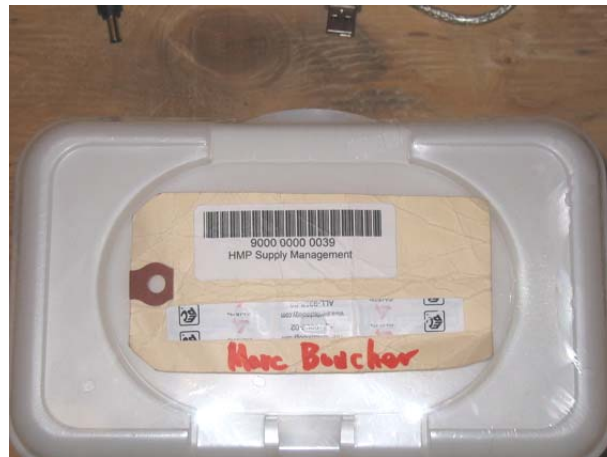
Figure 5.7: Example of a passive RFID tag and associated bar-code handed out to each HMP participant for the RFID gate experiment.
