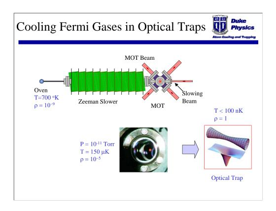
Our approach to producing a degenerate, strongly interacting gas differs from that of most other groups, in that we employ all-optical trapping and cooling methods. The optical trap is loaded from a standard magneto-optical trap which is produced from a slowed atomic beam.
