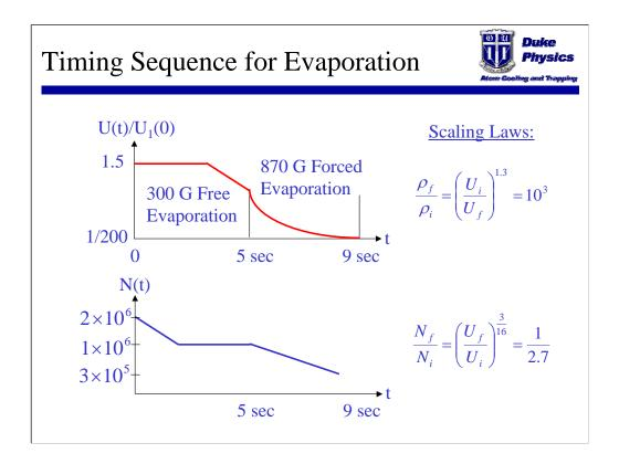
First, a 300 G magnetic field is applied at fixed trap depth. Then the trap is lowered at a field of 870 G, near the Feshbach resonance to produce a degenerate sample in a few seconds. Typically 2 million atoms are loaded. After free evaporation, 1 million atoms remain. Finally, after forced evaporation the number of atoms is reduced by a factor of 3, to 300 thousand, consistent with a scaling law model we have developed.
