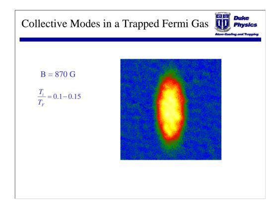
After the breathing mode is excited, the gas is held for a variable time, and then allowed to expand for 1 ms, after which it is imaged to show the oscillation.
