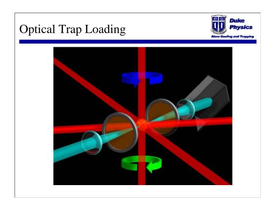
To reiterate the loading procedure, the  $\mathrm{CO}_2$  laser trap is first loaded from a magneto-optical trap. To increase the loaded number of atoms, the  $\mathrm{CO}_2$  laser beam is retroreflected using a rooftop mirror.
