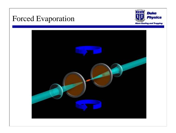
Next, the optical beams are extinguished and a magnetic field is applied to tune the gas into the Feshbach resonance region. Forced evaporative cooling is accomplished by lowering the trap laser intensity.
