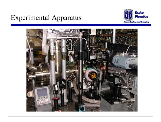
The lens in the foreground is used to focus the  ${\rm CO_2}$  laser beam into the vacuum system. A camera is used to record absorption images of the cloud.
