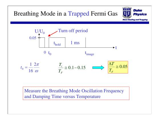
To avoid issues of deforming the Fermi surface in observing hydrodynamic expansion, we have instead measured the radial breathing mode frequencies and damping times. The breathing mode of the trapped gas is excited by briefly turning off the trap. The corresponding energy input corresponds to 0.05 TF when the trap is extinguished for 1/16 of a radial oscillation period, and is reduced to 0.01 TF when the trap is off for only 1/32 of a period.
