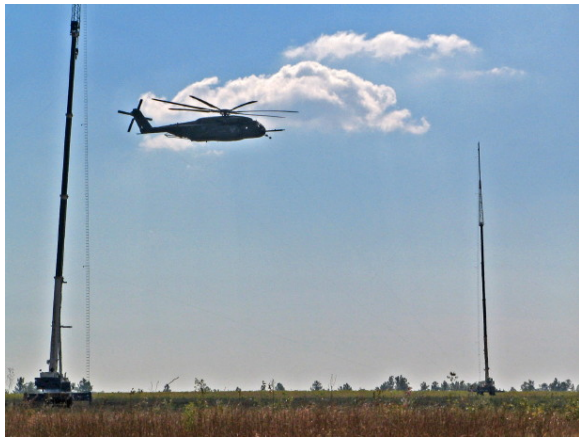
Figure 9. Photo of MH-53E flying through the goal-post microphone array.
