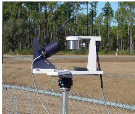
Figure 2. MultiFilter Rotating Shadowband Radiometer.
