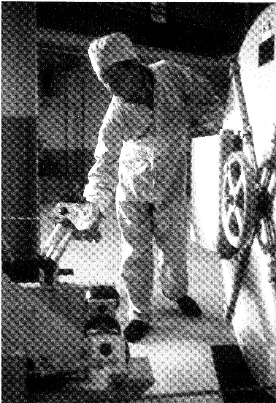
A health physics technician uses a handheld "curie pie" radiation detector to check equipment for contamination. (NASA C-2003-840)
