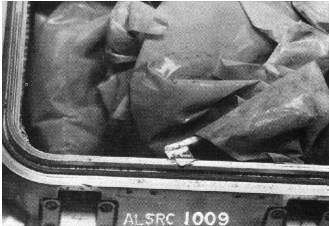
Figure 17. SRC 1009 indium seal from Apollo 16 (NASA photograph S72-37750).
