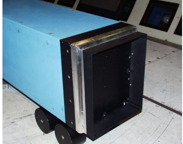
b) Shortened with fillets ( \Delta \bar{C}_D = -0.0573 )
