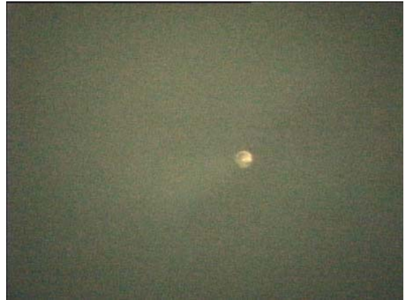
Fig. 3: An image taken from the rear surface of the aerogel tile from Shot 2 (magnification: 56×). The well-preserved spherical glass projectile was about 1 mm below the surface.
