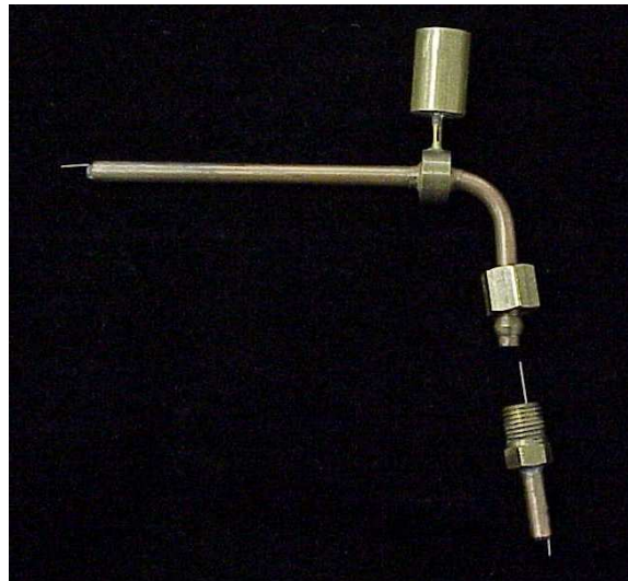
Figure 2.21. ‘L’ shaped smoke-wire holder/fluid applicator.
