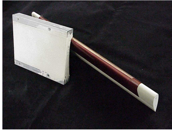
Figure 2.13. Airfoil with Kapton actuator at leading edge and template.
