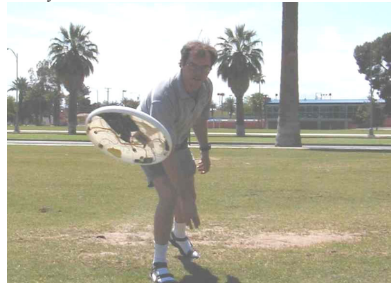
Figure 1. Test site and launch configuration. Note the high angle of attack of the disc.
