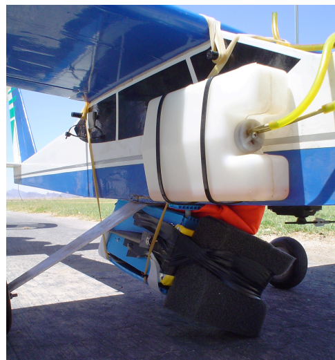
Fig. 3. Upclose view of the first probe under the fuselage with the medium-sized, flat parachute.
