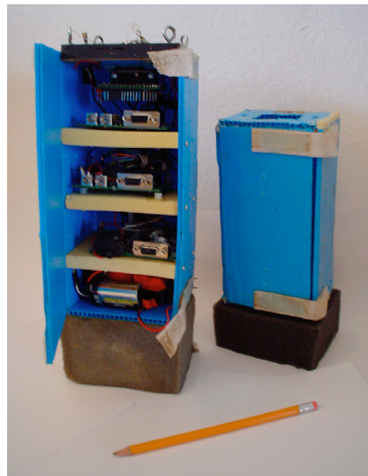
Fig. 1. The two versions of the parachute-probe dynamics test-beds with a pencil for size reference. The preliminary version, shown on the right, was soon replaced with the larger version, on left, to better support the growing sensor package.
