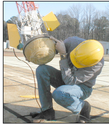
Fig. 8. Impact Absorber, Post-Test
