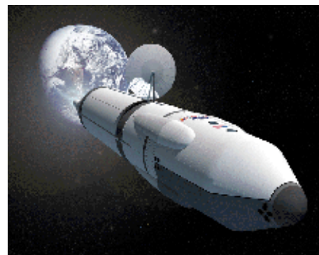
Fig. 1. Nuclear Thermal Rocket/Mars Aerocapture Vehicle leaving Low Earth Orbit. The Apollo shaped cap on the front served as the Earth Return Vehicle in the mission study [3,4].
