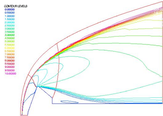
Fig. 15. Computed Mach Number contours for axisymmetric Mach 10, 70^\circ Sphere-Cone of Hollis and Perkins (from [42]).
