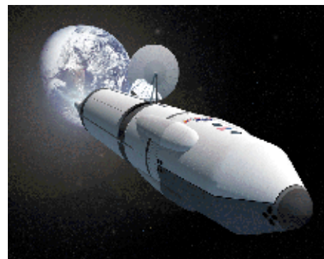
Fig. 1. Nuclear Thermal Rocket/Mars Aerocapture Vehicle leaving Low Earth Orbit. The Apollo shaped cap on the front served as the Earth Return Vehicle in the mission study [3,4].
