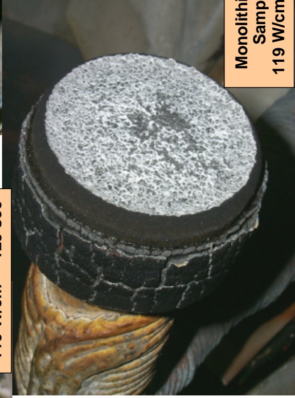
Strip-Collar Bonding Sample 3085 119 W/cm 2 – 125 sec
