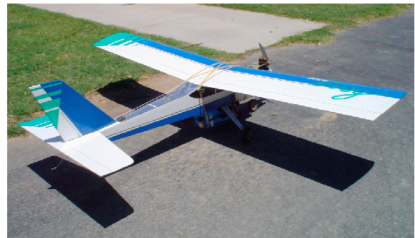
Fig. 2. The Xtra-Easy airplane taxiing to the runway with the probe and parachute securely mounted under the fuselage.
