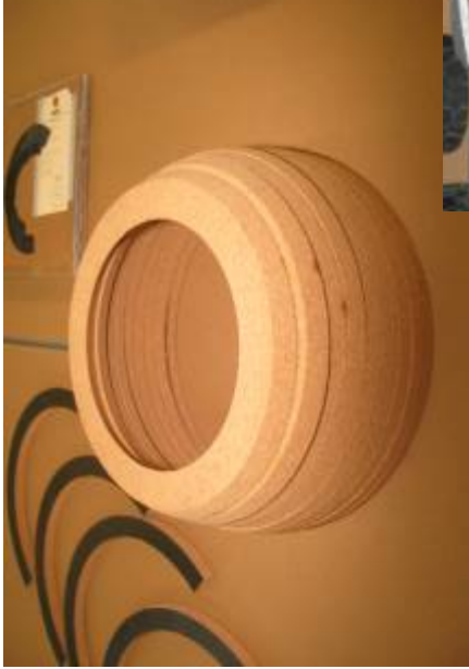
Slices of ablator material ready for assembly into sub-scale ellipsoidal heatshield
