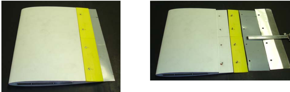
(a) (b) Figure 2. (a) NACA0012 airfoil model with a Mylar SETE, (b) Baseline model, removable parts, and aluminum SETE and Mylar SETE.
