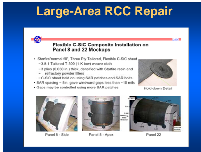
Figure 48. Demonstration of large area repair (LAR) concept and attachment means to repair a RCC wing leading edge.
