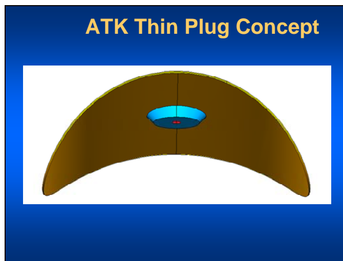
Figure 44. Final design of the “new” ATK Thiokol thin, flexible C-SiC plug for RCC repair.
