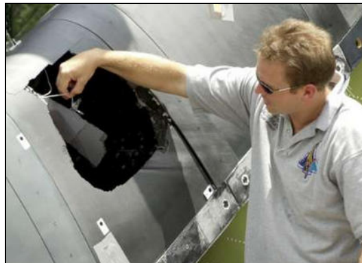
Figure 5. Large hole in panel 8 post test at Southwest Research Institute (SwRI).
