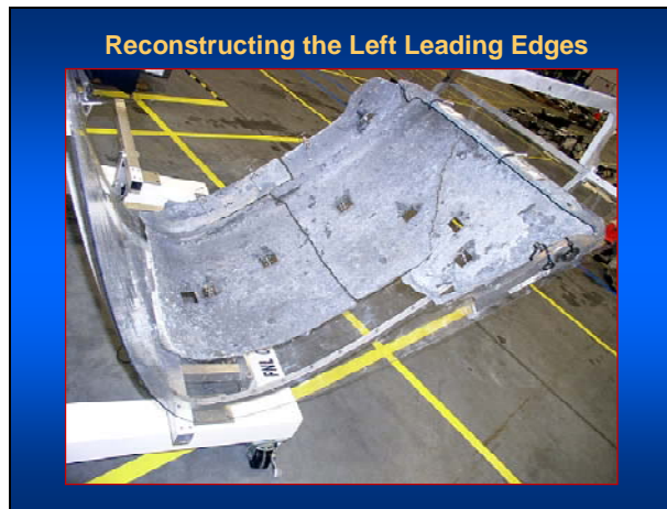
Figure 4. Inner surface of port wing RCC leading edge panel with thin metal coating believed to be deposited during hot gas ingress to the wing cavity.
