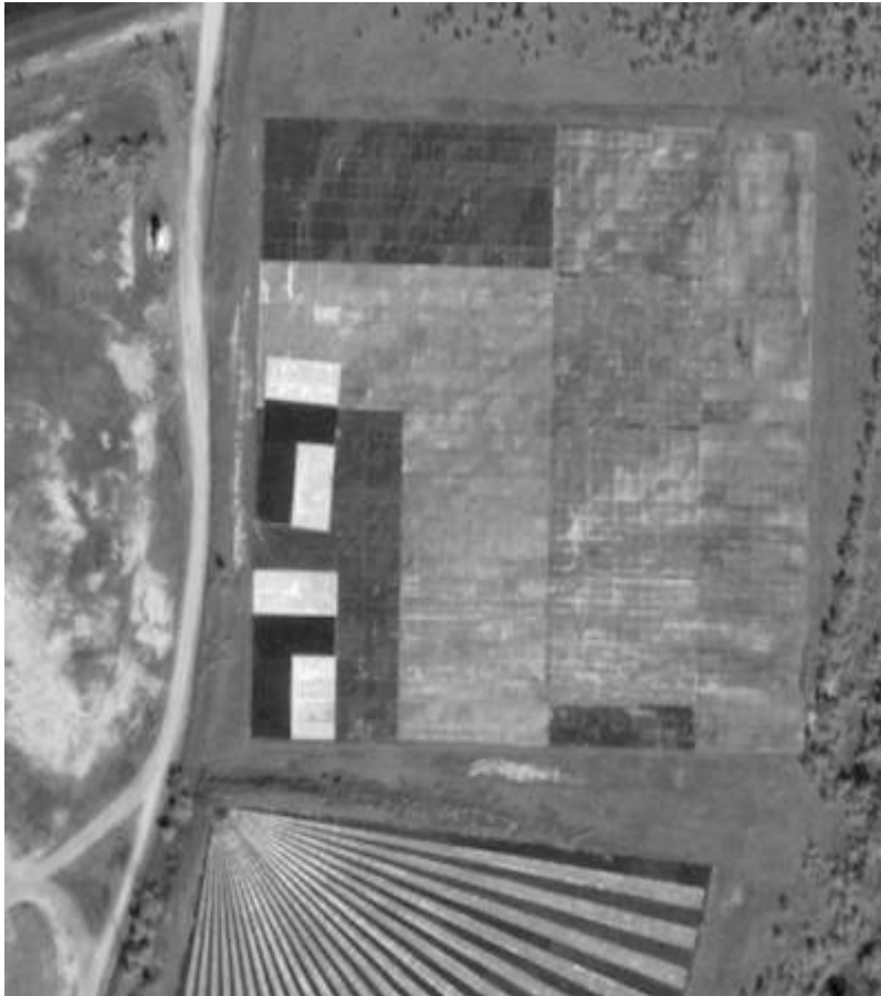
Image of the SSC edge targets acquired by the QuickBird satellite (60 cm GSD).
