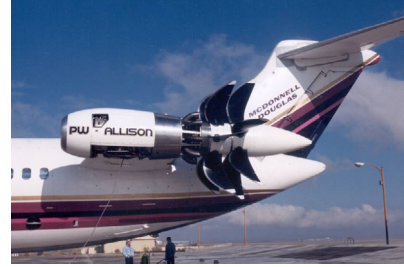
Figure 4.—Ultra-high bypass ratio propulsors designed, built, and flight tested.
