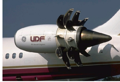
Figure 4.—Ultra-high bypass ratio propulsors designed, built, and flight tested.
