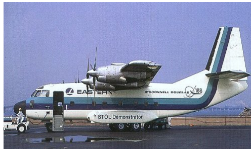
Deflected Slip Stream Turboprop
