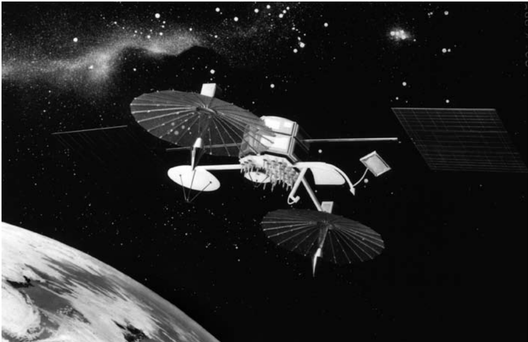
A drawing of the TDRS-3 spacecraft. The Tracking and Data Relay Satellite System (TDRSS) provides nearly uninterrupted communications with the International Space Station (ISS), the Space Shuttle and Earth orbiting satellites, replacing the intermittent coverage provided by the Spaceflight Tracking and Data Network (STDN) ground stations. (NASA Image Number MSFC-8893551)
