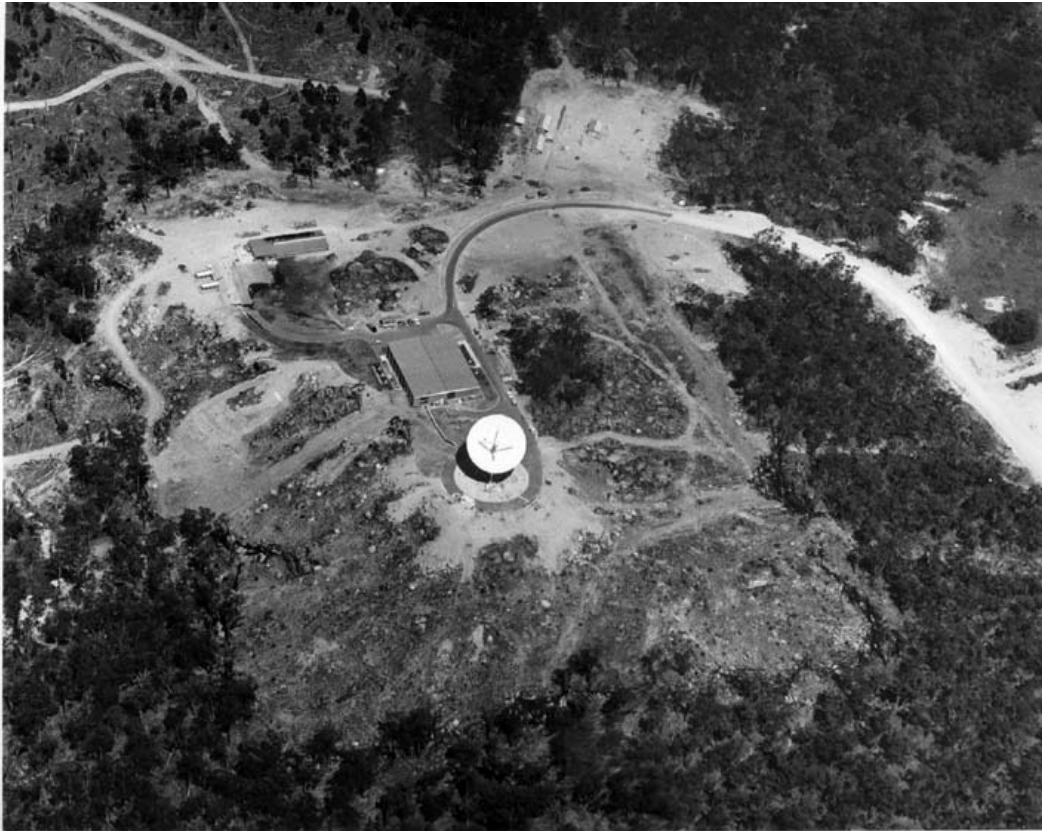
Aerial view of the Apollo Station at Honeysuckle Creek, Australia with its 26-meter (85-foot) Unified S-Band antenna. At the upper left are the diesel fuel tanks for the power generators. Because of its remote location in a national forest, this crucial Apollo Station was run entirely off generator power. (Un-numbered photograph, Box 18, NASA Australian Operations Office, Yarralumla, ACT)
