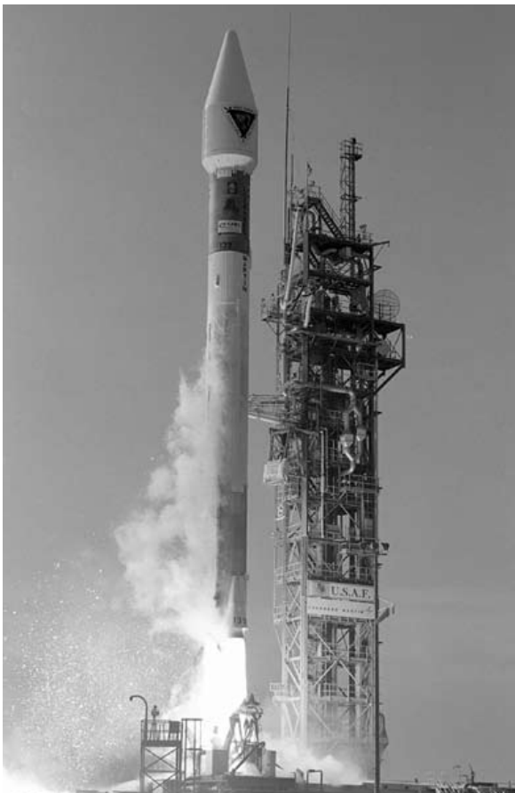
Unlike the first generation of Tracking and Data Relay Satellites, TDRS-H, I and J were launched using expendable launch vehicles. Here, TDRS-H rises from PAD36A, Cape Canaveral Air Force Station at 8:56 a.m. EDT on 30 June 2000 atop an Atlas IIA/Centaur launch vehicle. The new satellites augmented TDRSS's existing S- and Ku-band capabilities by adding a Ka-band capability. (NASA Image Number KSC-00PP-0825)
