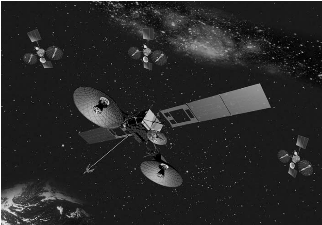
Artist rendition of a Tracking and Data Relay Satellite providing communications support from Earth orbit. The long and winding road has taken NASA’s Spaceflight Tracking And Data Network from a handful of ground stations in the late 1950s to the Space Network of the twenty-first century. (NASA Lithograph LG-2001-8-033-GSFC)
