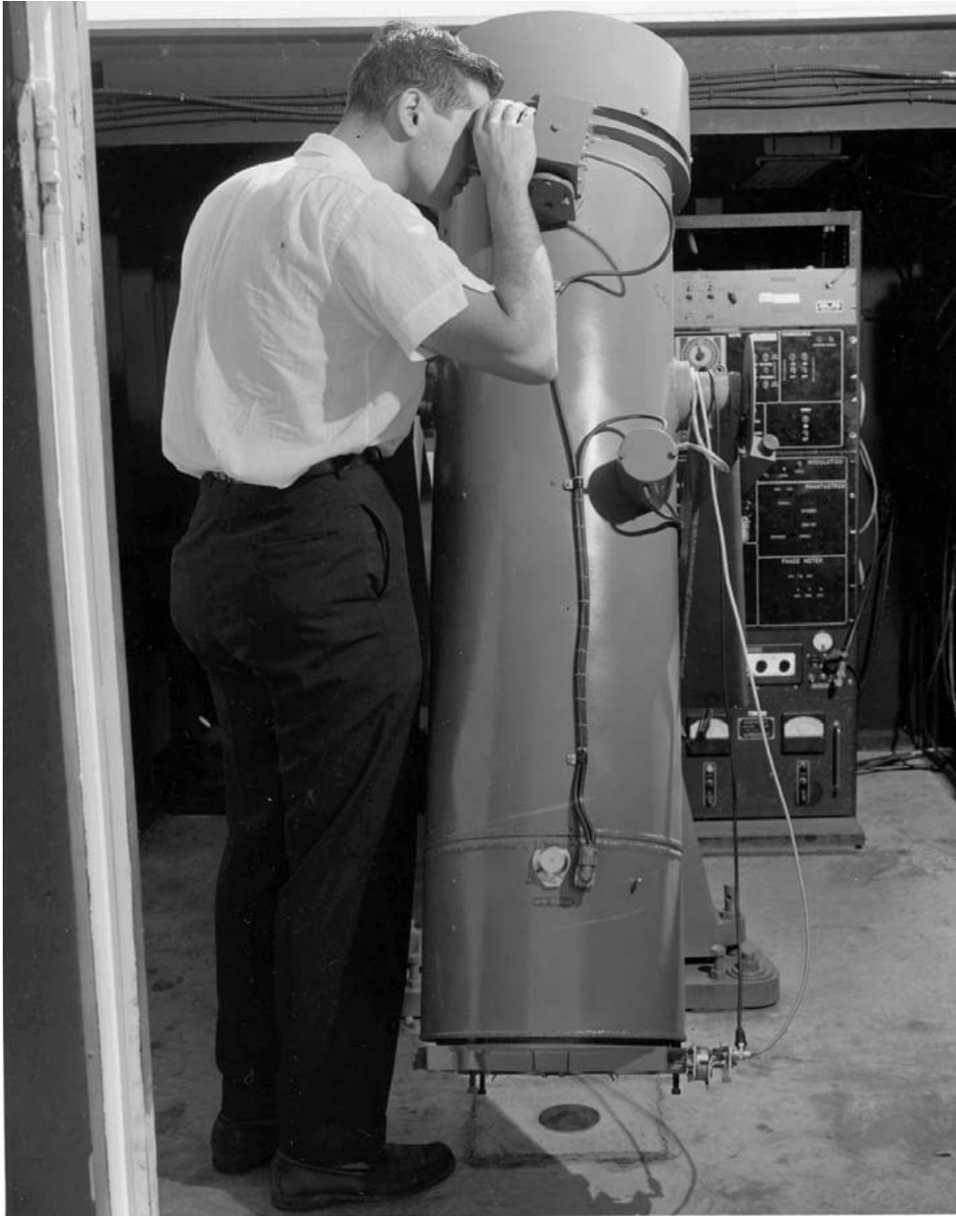
One of the lesser-known tracking systems developed by GFSC was the MOTS—Minitrack Optical Tracking System—which was used to obtain precise, position calibration and misalignments in the Minitrack system. The photograph shows David W. Harris (who later became a Deputy Associate Administrator at NASA Headquarters) operating the camera at Blossom Point in 1963 after it was modified to photograph passive satellites such as Echo. Note the photographic plate at the bottom of the camera. MOTS was used until the 1970s. (NASA Image Number G-63-826)
