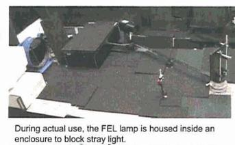
During actual use, the FEL lamp is housed inside an enclosure to block stray light.
