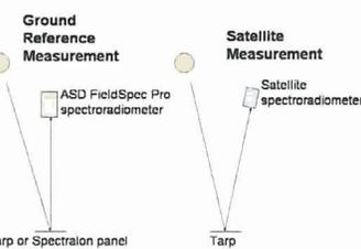
In general, satellite is not at zenith, and plane of reflection is not at same azimuth as plane of incidence.
