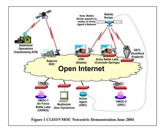
This network was configured exclusively for IPv4 networking. IPv4 static routing and IPv4 mobile networking capability were configured in the network infrastructure. No IPsec for IPv4 or IPv6 capabilities were turned on, even though those capabilities were already present onboard CLEO in its copy of Cisco's Internetworking Operating System (IOS), as the ground infrastructure being tested for VMOC and the SSTL ground networks did not support IPv6 at that time.
