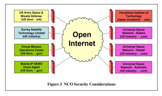
Glenn Research Center's (GRC's) network is a localized research network directly connected to the open public Internet and isolated from the GRC operational network. Likewise, the US Army Space and Missile Defense network is an experimental network isolated from any operational networks.
