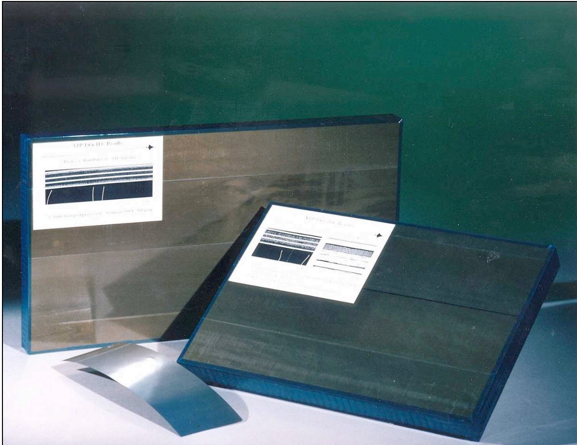
Figure 37 – TiGr honeycomb laminates made by interleaving titanium and IM-6/PEEK plies using the primary bonded honeycomb process.
