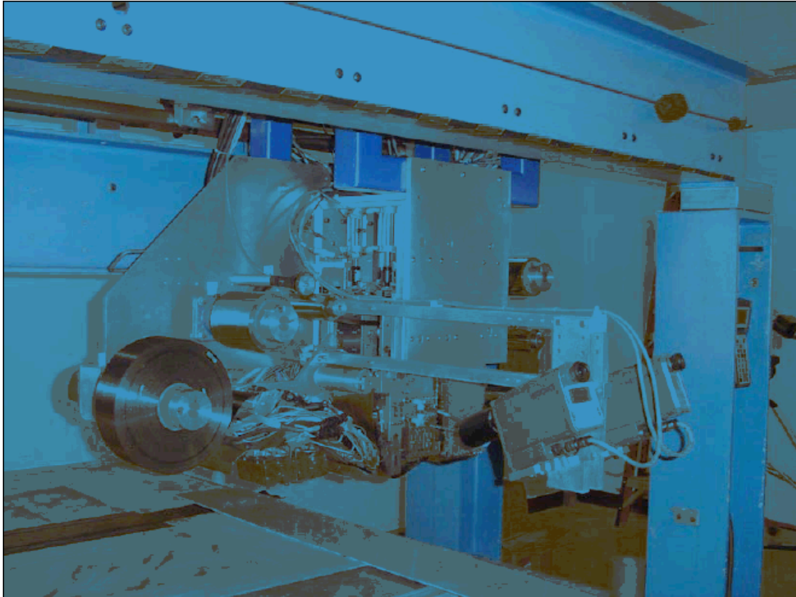
Figure 40 – Accudyne Systems installed a heated thermoplastic deposition head at NASA-LaRC. The head consolidates thermoplastic tape into a laminate using Accudyne’s in- situ consolidation process. The head’s three conformable compactors allow fabrication of laminates with complex curvature.
