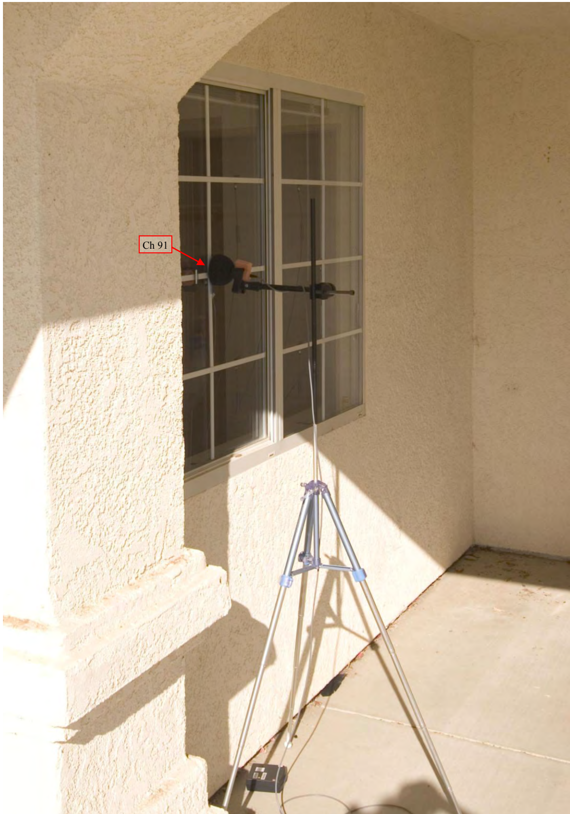
Figure 3.9: Typical exterior window near-field microphone. Microphone and windscreen were held in a holder mounted to a tripod. Channel 91 is shown.
