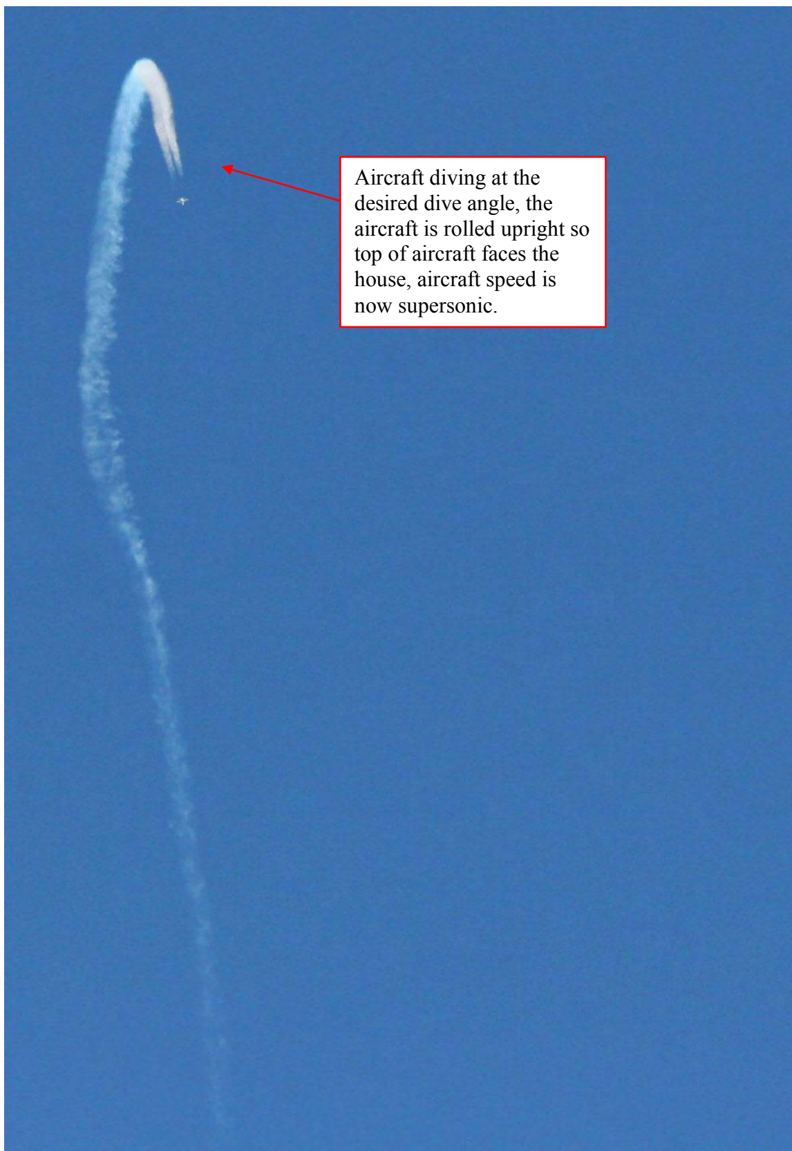
Figure 4.2: F/A-18B aircraft is rolled upright while in a dive at an angle of 53 degrees.
