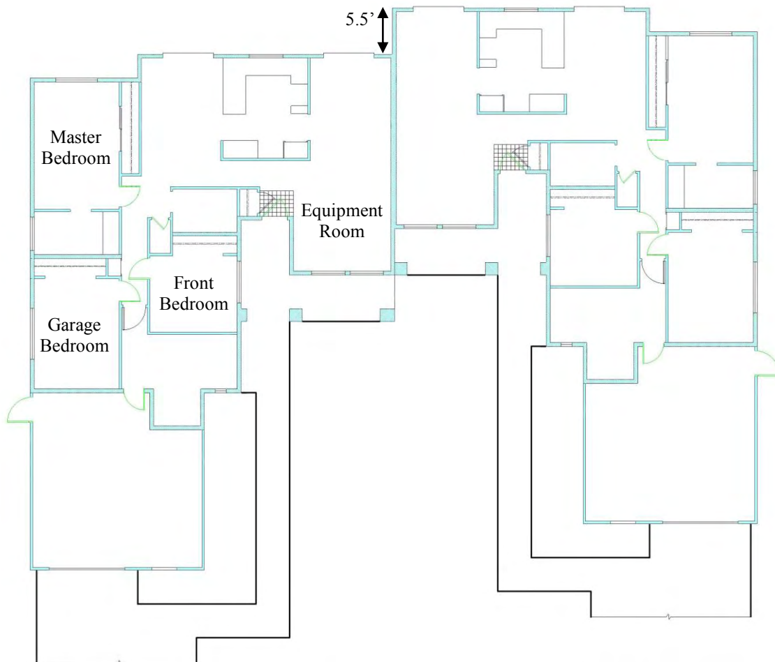
Figure 2.3: Floor plan of the duplex illustrating both sides of the house. The floor plans are mirror images of each other, offset by 5.5 feet.
