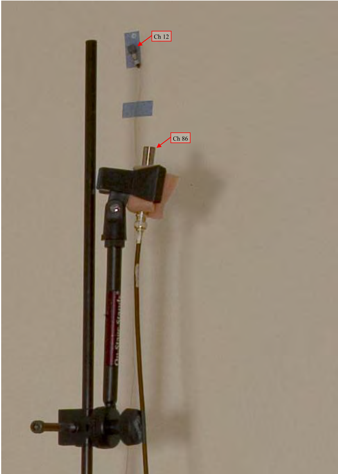
Figure 3.7: Detail of a typical indoor microphone mounted in a holder. Channel 86 is shown.
