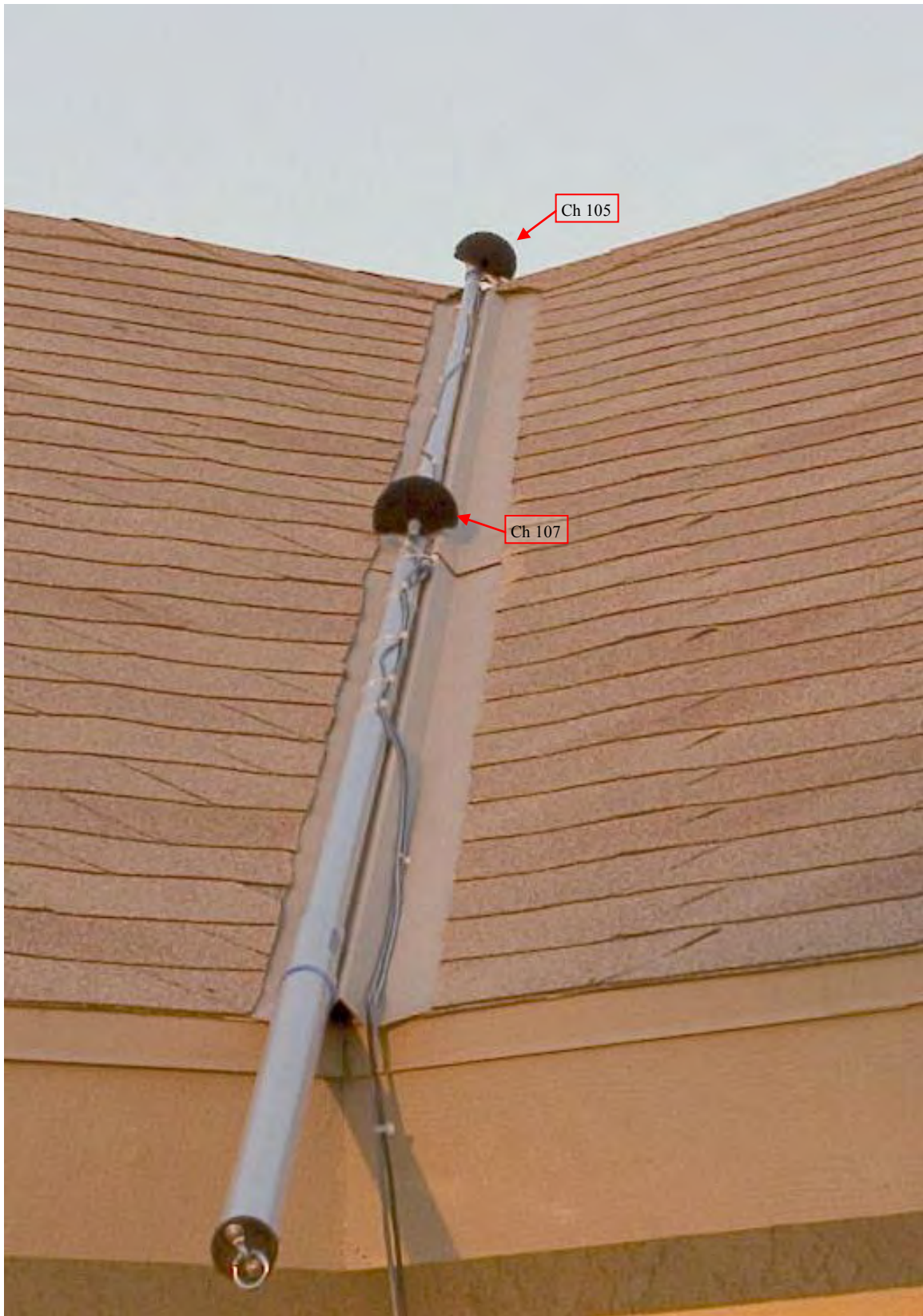
Figure 3.11: Exterior rooftop microphones mounted to a pole for easy installation. Channels 105 and 107 shown.
