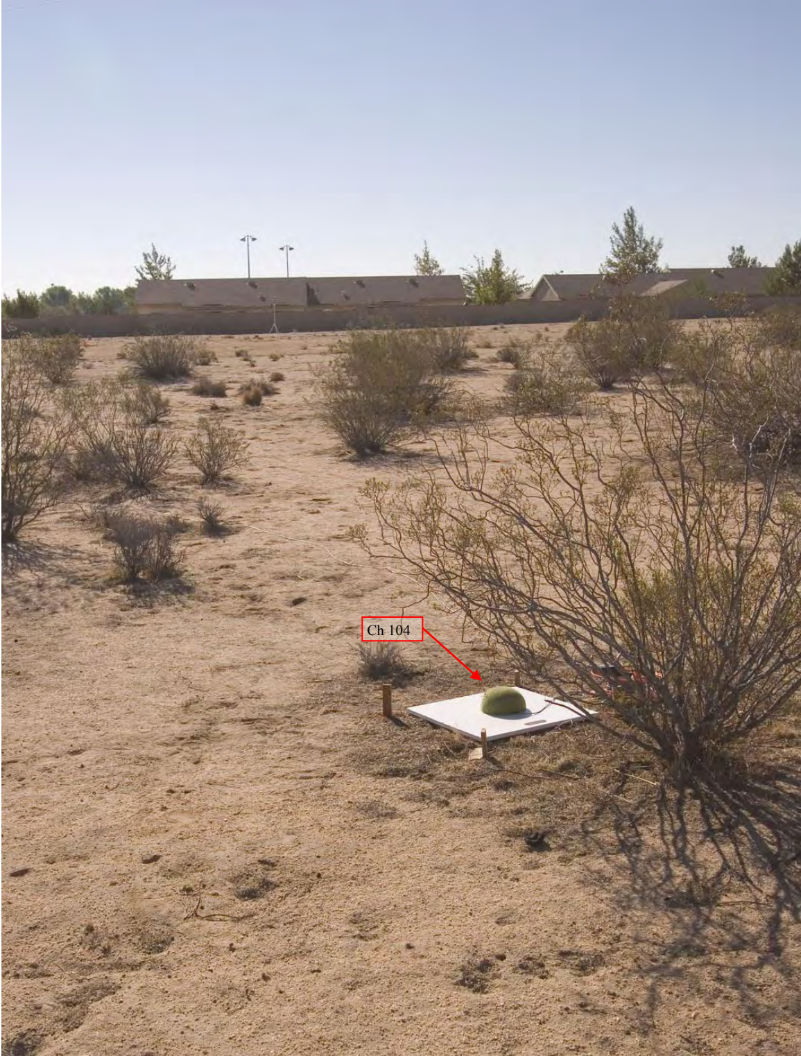
Figure 3.13: The far field microphone.
