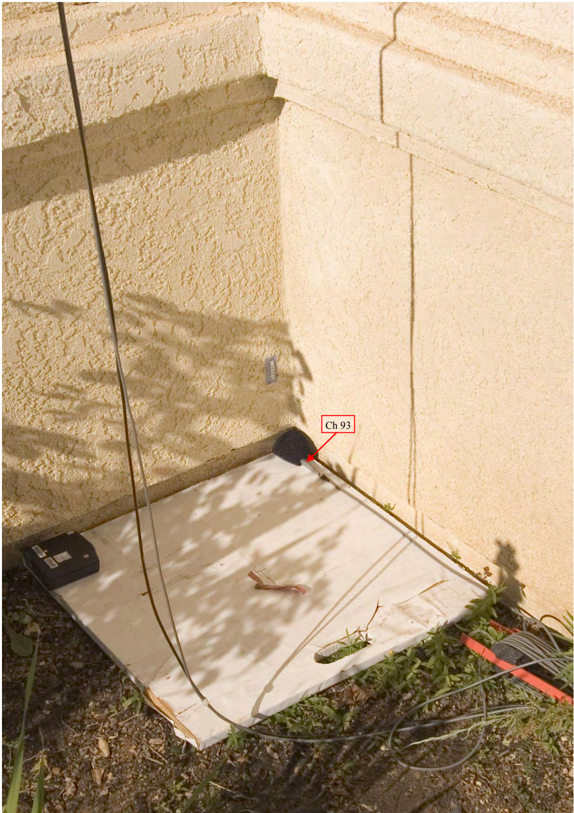
Figure 3.12: Typical exterior ground microphone. Channel 93 shown.
