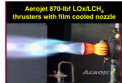
Aerojet 870-lbf LOx/LCH 4 thrusters with film cooled nozzle
