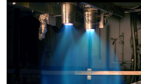
Dual 870-lbf LOx/LCH 4 thrusters with ablative nozzles in WSTF APSTB
