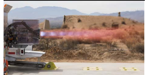
KTE LOx/Methane workhorse main engine installed at MSFC TS500
