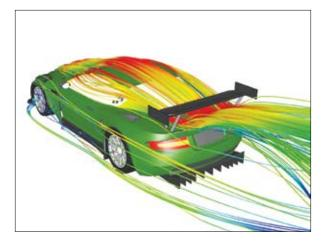
Computational fluid dynamics (CFD) is proving an effective method for testing racecars—replacing, in some instances, the traditional track and wind tunnel tests.
