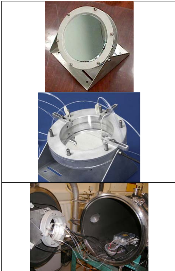
Figure 4. The front (top) and back (middle) views of a prototype FOMIS unit. The bottom image shows the unit and the electronics inside the two-stage light gas gun test chamber at Kent. Right before the closing of the chamber, the unit was turned 180° to allow the front side to face the incoming projectile.
