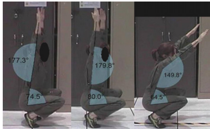
Fig. 2. Example: Posture while crouching and reaching overhead in oversized (Left), appropriately Sized (Center) and undersized (Right) Flight Suits
