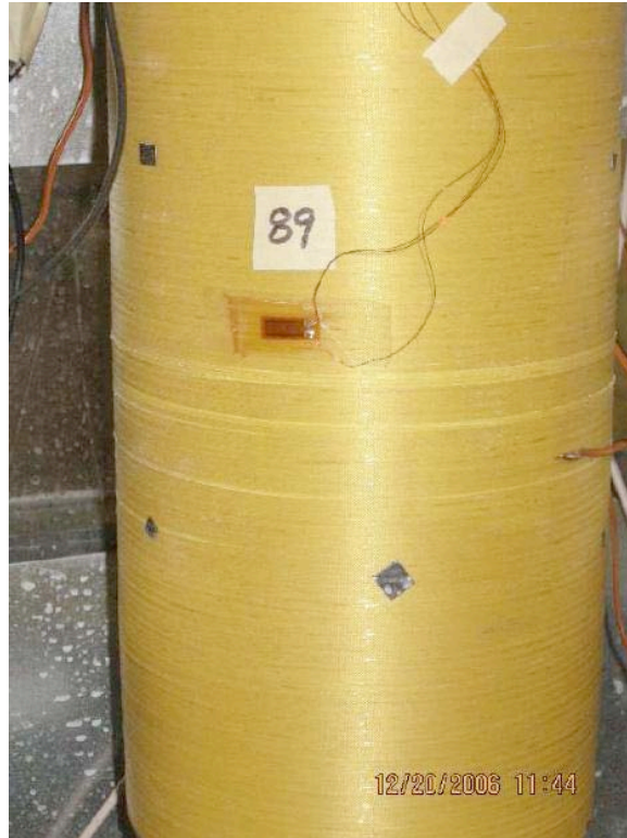
Figure 2: COPV pulled before failure due to Fiber damage.
