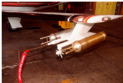
Attached to the wing of a Cessna Citation aircraft are cloud physics probes that measure the size, shape and number of ice and water particles in clouds. The plane is also equipped with field mills, used to measure electric fields. The plane was flown into anvil clouds in the KSC area as part of a study to review and possibly modify lightning launch-commit criteria.
