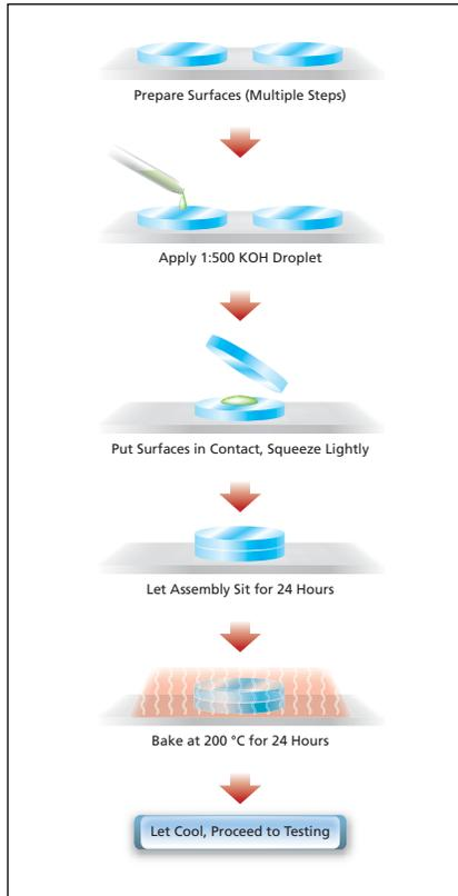
Two Prepared Surfaces are placed in contact with a small amount of a hydroxide solution at the interface. The assembly is allowed to sit and is then baked. The resulting bond is at least as strong as an epoxy bond.
