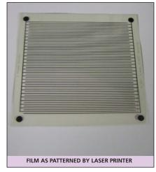
A Pattern of Interdigitated Electrodes was formed directly on the ITO-coated surface of a transparent polyester film by use of a laser printer. After etching away of the ITO not covered by the toner, the toner was washed away, leaving the polyester film with the patterned
