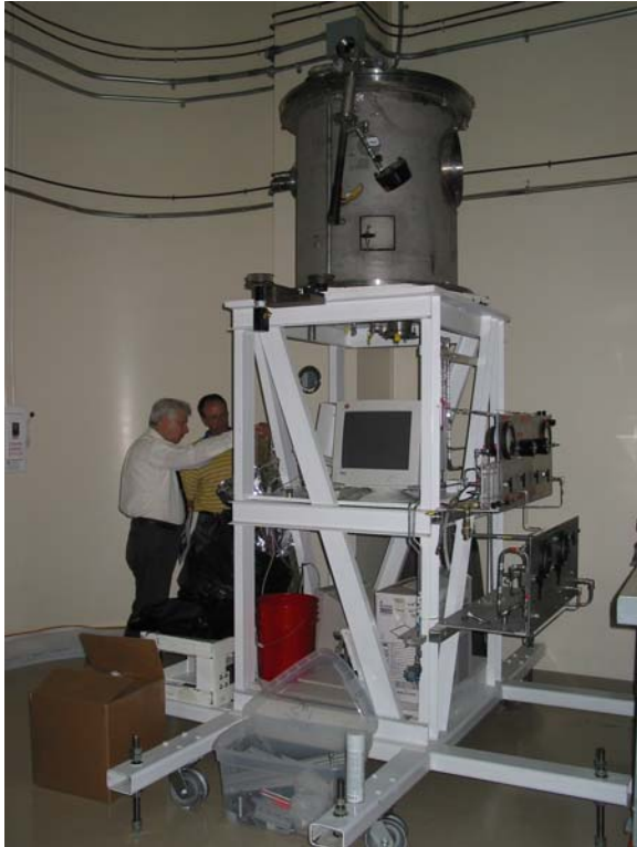
Figure 3. IHRPT Solar Concentrator System Ground Demonstrator base and vacuum chamber.
