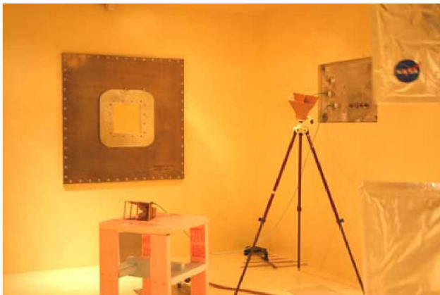
Figure 1. Composite Panel Mounted in Test Fixture
