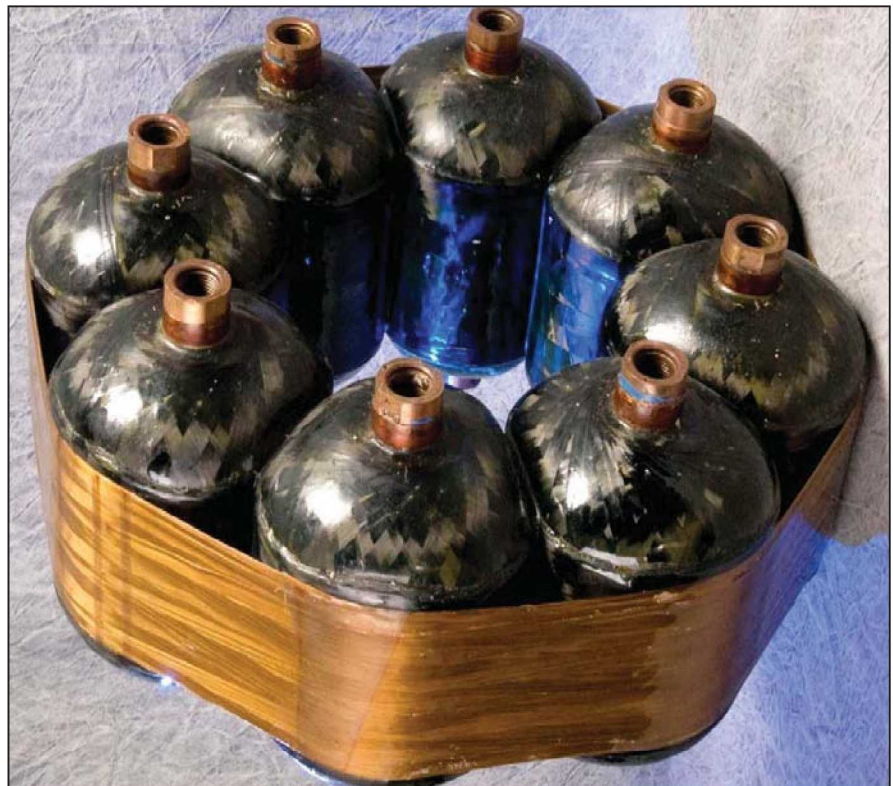
This Prototype Assembly of Conformal Tanks was built to demonstrate the feasibility of building such an assembly to fit an approximately toroidal available volume.
