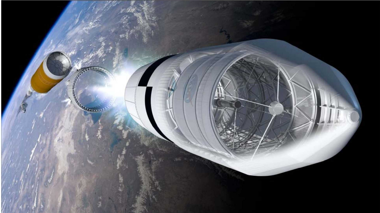
Figure 8: Artist's concept of the Ares V launch of an 8-meter monolithic telescope visible in the cutaway depiction of the payload shroud
