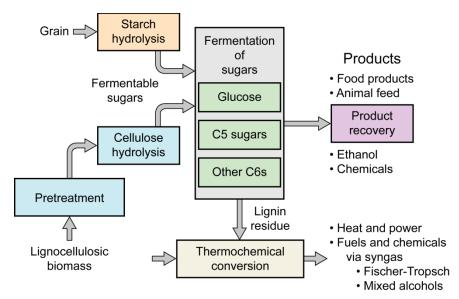
Figure 3.—Conceptual example of processing of biomass at biorefinery (Ref. 32).
