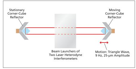
**Displacement Oscillations** are introduced between two corner-cube retroreflectors that are common to two displacement gauges. The magnitude of an amplitude modulation in the outputs of the gauges is measured.
